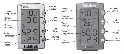
The POWER button turns the display on and off. The display draws 35 mA when on and .3 mA when off. The display is equipped with a backlight for low-light conditions. Enable the backlight by pressing the UP arrow or turn the backlight off by pressing the DOWN arrow. The model X4D has three levels of backlighting.
