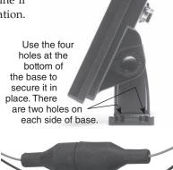
Pull rubber fuse housing apart to access fuse.
